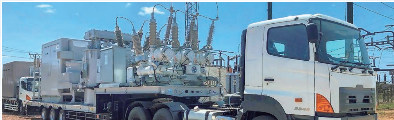
66/33kV Mobile Substation (20MVA)
