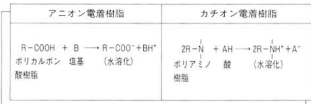
図2 / アニオン電着塗料とカチオン電着塗料の比較 Fig. 2 Comparison between anionic electrodeposition paint and cationic electrodeposition paint
