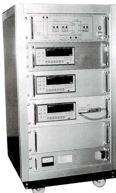
図7/巻線抵抗測定装置の外観 Fig. 7/Measuring equipment for winding resistance
